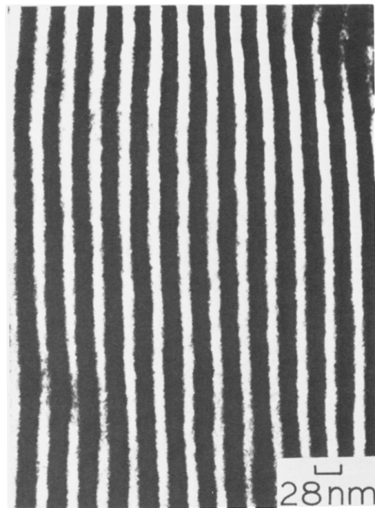
Figure 18. Bright-field (BF) image of osmium tetroxide stained ISI lamellar copolymer (dark, isoprene; light, styrene).
